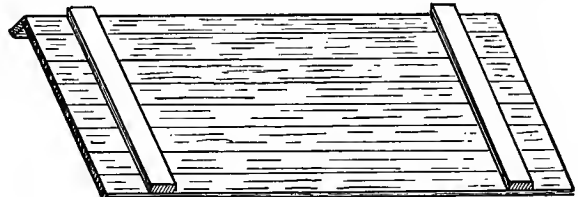
FIG. 43. A DROPPINGS' BOARD (INVERTED) Showing how the match-boarding should be braced underneath, and the droppings' board fitted with a ledge in front
