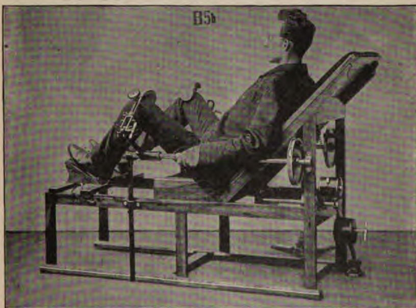
Fig. 4a.—Zander Vibrator Massage Apparatus Showing Method of Operation.
