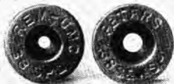
An extreme example in variations in vent sizes as described on page 60.
