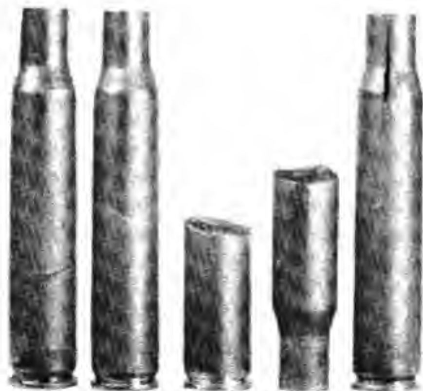
Split and ruptured cartridge cases.
