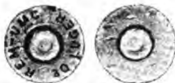
These cartridges fired prematurely from the slam of the breech block because the primers projected slightly above the case heads. Note the mark of the firing pin hole and the absence of firing pin indentation.
