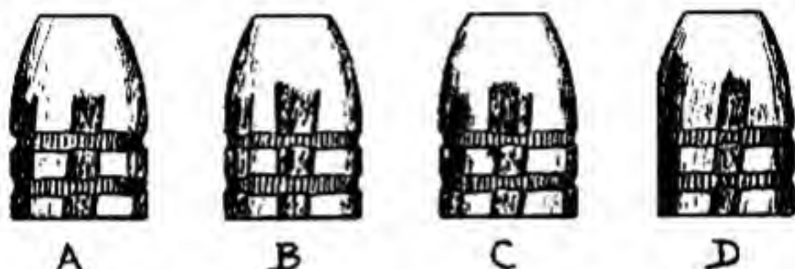
Results of slippage, tipping and shaving of bullets.
