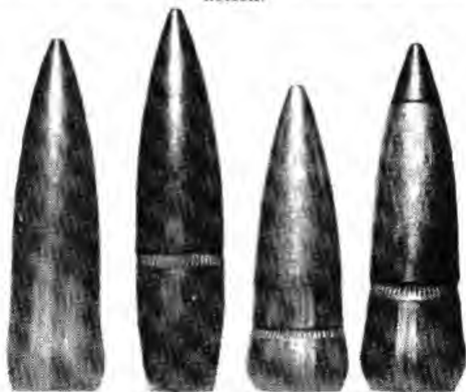
Showing upsettage of bases of flat base bullets in comparison with a boat-tail bullet which does not upset when fired. Upsettage depends upon the structure of the bullet, its hardness, the force applied behind it and the suddenness with which the force is applied.
