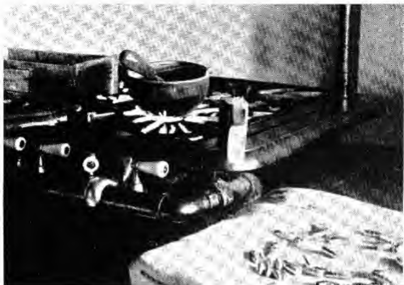
Usual "set-up" for proper casting of bullets over the gas range.
