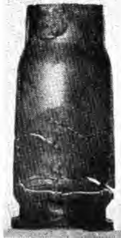
An automatic pistol case which has been fired to destruction with mercuric primer. Originally fired with a mercuric primer, it was then reloaded and fired three times with non-mercuric primers—with the result shown above.
