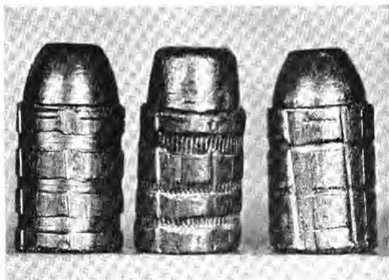
The difference between well and poorly designed lubrication grooves and properly sized bullets is not always apparent until after the bullet has been fired. The bullet on the right has its grooves practically closed up.
