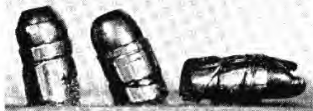
Hollow base bullets in which the cavity was carried too deep. When fired, the bullet slugged badly or the base blew out and the sides collapsed.
