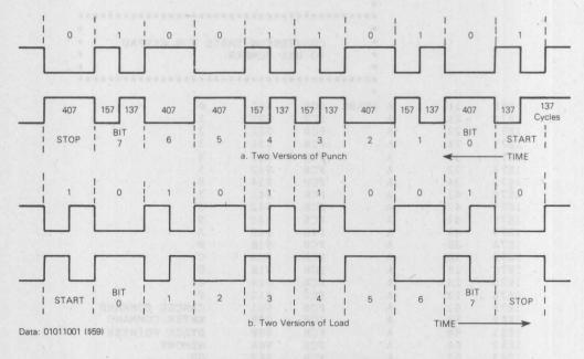
Figure 9. Example of Serial Data Formats for Punch and Load
