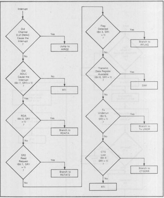
Figure 9. Flowchart of DMA-ADLC Program (Sheet 3 of 9)
