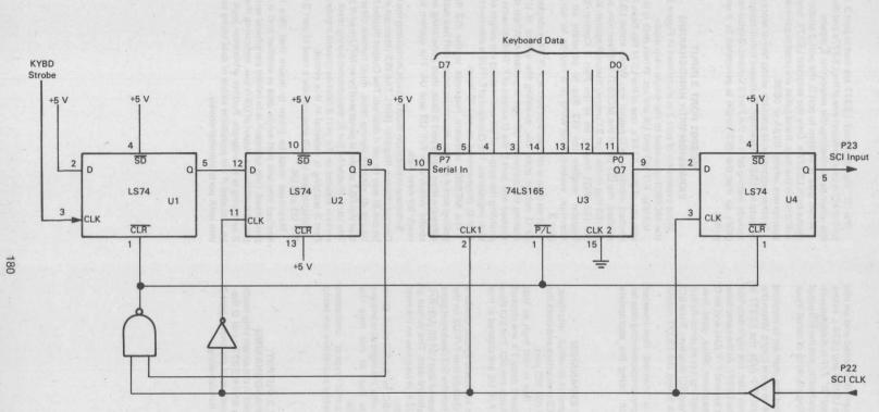
FIGURE 4 - SCI Keyboard Interface
