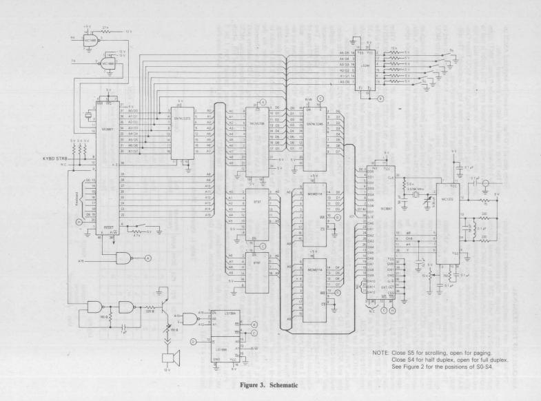
The VDG outputs chrominance ( $\phi A$ ,  $\phi B$ , Y) and chroma bias (CHB) to the MC1372 Modulator which generates composite video for the television. The Modulator is clocked by a 3.58 MHz crystal and its TTL compatible clock output (pin 1) is used to drive the VDG.
