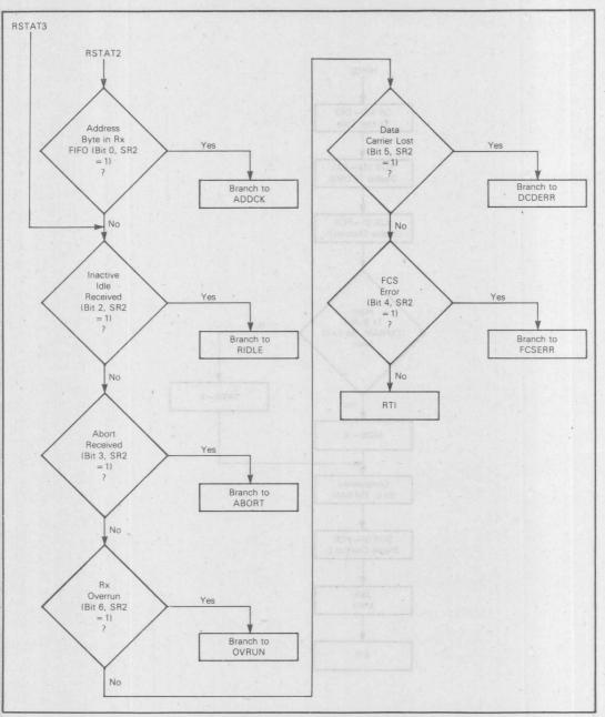
Figure 9. Flowchart of DMA-ADLC Program (Sheet 5 of 9)
