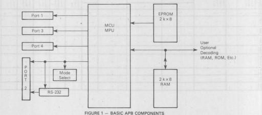
the monitor ROM features in LILbug<sup>®</sup>. Thus, the APB together with LILbug provides features which allow the user to: (1) Develop and edit software programs; (2) Hardware trace through the user's program; (3) Insert, display, and remove breakpoints in the program; and (4) Provide punch, load, and verify commands for software I/O. To utilize the ROM features in LILbug, the MC6801L1 MCU must be used.
