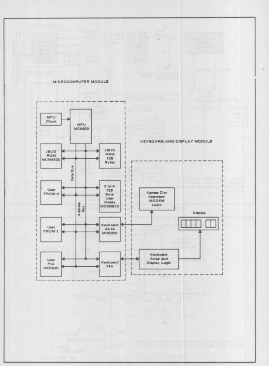
FIGURE 1 - MEK6800D2 Block Diagram
