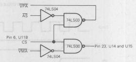
Note: When VMA is used, AS should be disconnected from the CS decoding (Figure 1, U11B) and that input is tied active.
