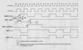
FIGURE 2 – MC6875 Interface Timing: Dynamic Memory Refresh
