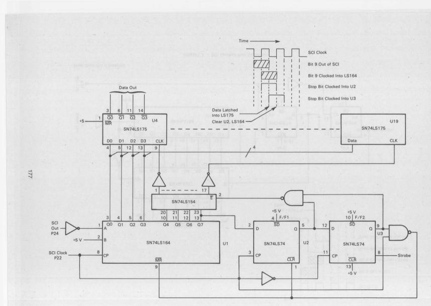
FIGURE 2 — Latched SCI Output Expansion
