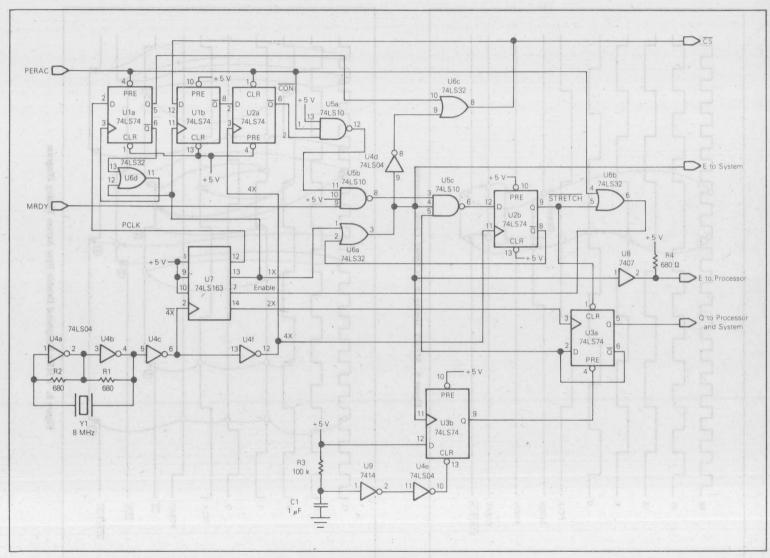
Figure 4. Clock Generator Circuit for MC6809E
