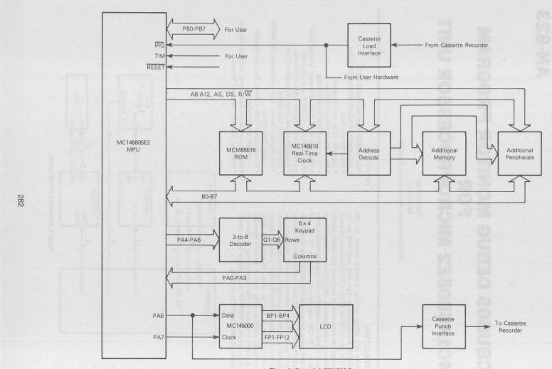
Figure 2. Expanded CBUG05 System
