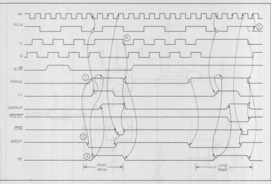
Figure 3. Half-Speed Circuit Timing
