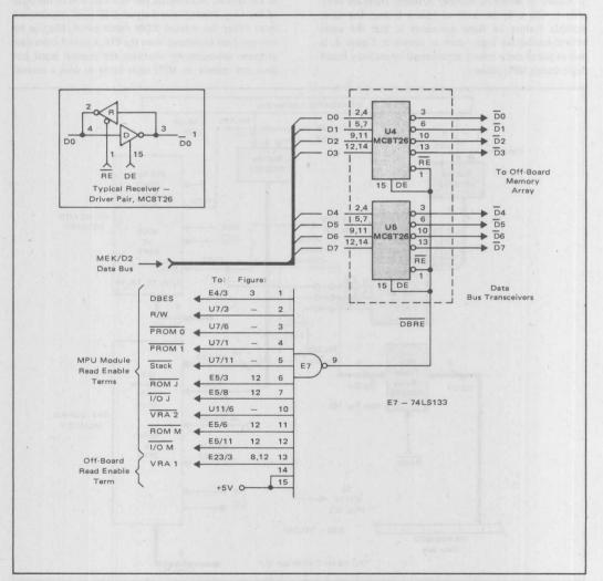
FIGURE 10 – Data Bus Expansion Control Logic
