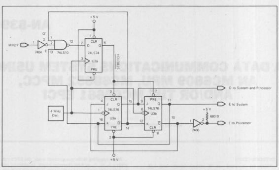
Figure 7. Clock Generator for MC6809E with MRDY Input
