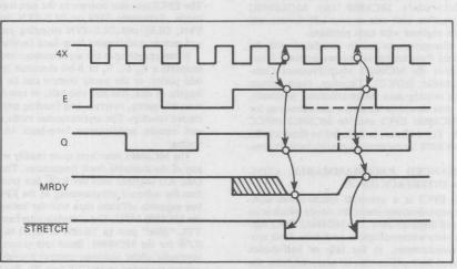
Figure 8. MC6809E Clock Generator Timing Diagram
