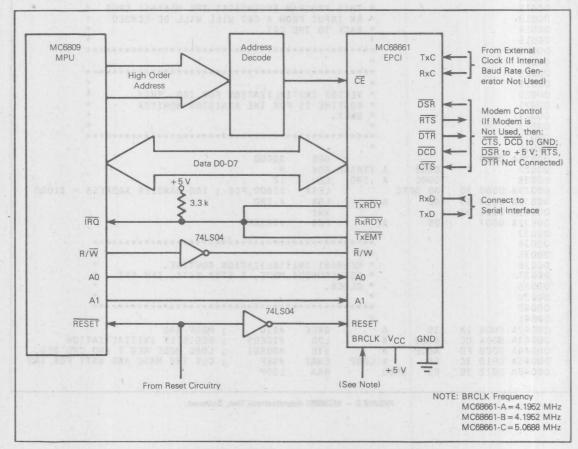
FIGURE 1 - MC6809 to MC68661 Interface Connection, Schematic Diagram
