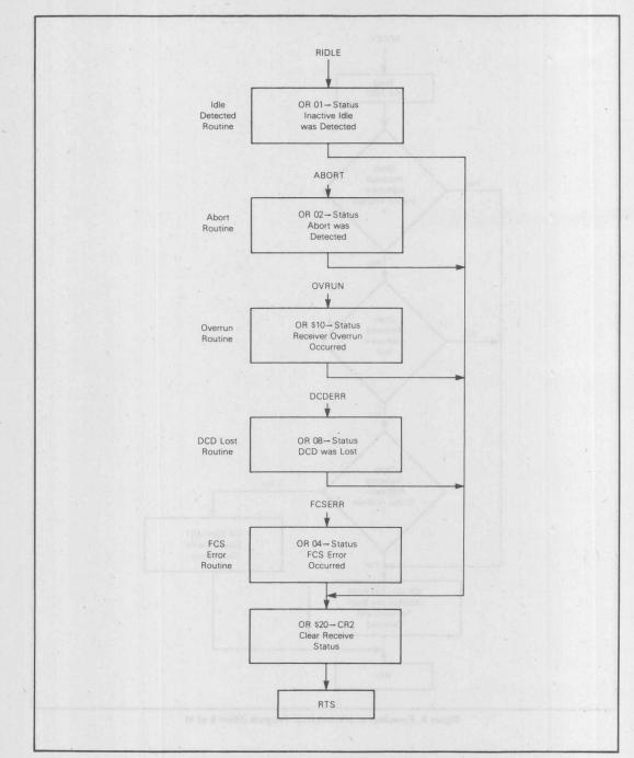
Figure 9. Flowchart of DMA-ADLC Program (Sheet 7 of 9)
