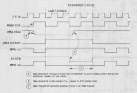
FIGURE 3 – MC6875 Timing: DMA (MC6844) Three-State Steal Mode
