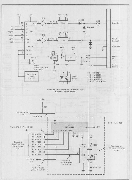
FIGURE 17 - Baud Rate Logic
