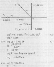
Step (5) - Filter Section Q and Center Frequency
