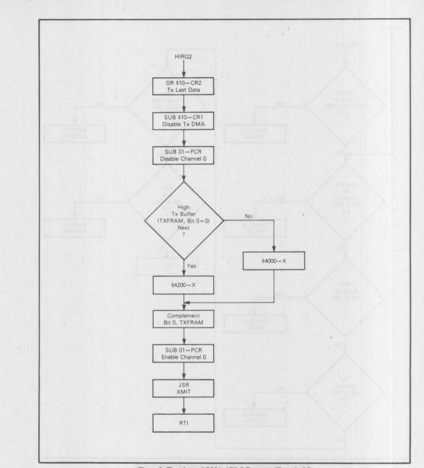
Figure 9. Flowchart of DMA-ADLC Program (Sheet 4 of 9)
