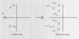
The bandpass filter will take on a form of three 2-pole bandpass filter sections in cascade. When bandpass sections are cascaded, each section center frequency and Q must be determined from the low pass damping factors ( $\xi$ ) and natural frequencies ( $\omega$ ).
