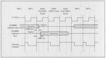
Figure 10. System DMA Cycle Timing
