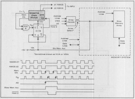
FIGURE 6 - Slow Memory Handshake Logic and Waveforms
