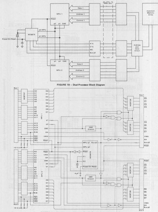
FIGURE 20 - Dual Processor (Multiplex Processing To Common Memory)
