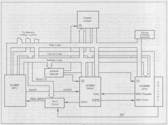
Figure 2. DMA System Block Diagram
