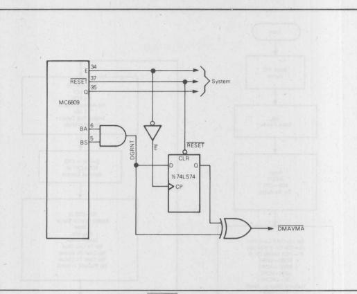
Figure 8. DMAVMA Generation Circuit
