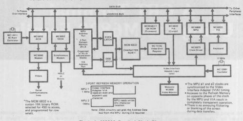
Figure 1. M6800 Terminal Block Diagram
