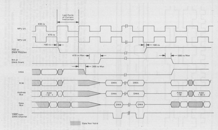
FIGURE 9 - Timing of DMA Transfers by Halting the Microprocessor
