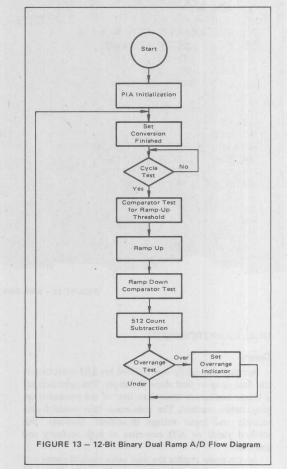
then stored back into the same memory location. Lines 86 and 87 check the contents of memory location TEST for a number greater than  $4095_{10}$ . If this condition occurs, the overrange, conversion finished, and ramp control bits are set high. Otherwise the MPU branches back to line 50 where only the conversion finished and ramp control bits are set high. The program then checks the status of the cycle input waiting for the next conversion.
