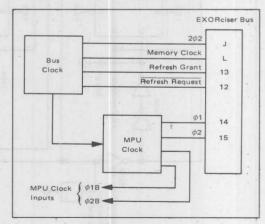
FIGURE 7 - System Clock Block Diagram
