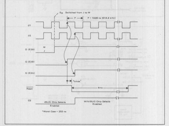
FIGURE 13 – Monitor Chip-Select Timing – Manual Select Select MINIBUG, Deselect JBUG
