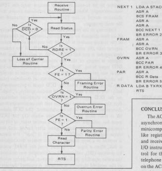
FIGURE 14 - Flow Diagram and Source Statements for **Receive Subroutine**
