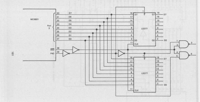
FIGURE 5 - MC6801 Port 3 Expansion (Output)
