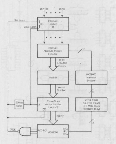
Figure 2. Vector Number Generation Circuit - Block Diagram
