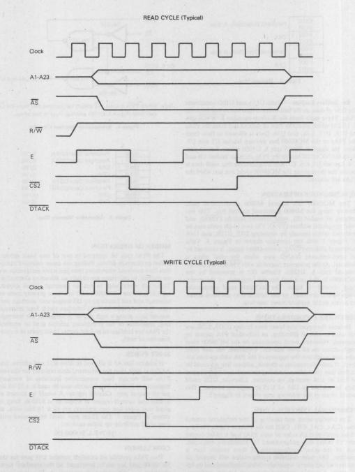
Figure 2. Asynchronous Interface Timing Diagrams
