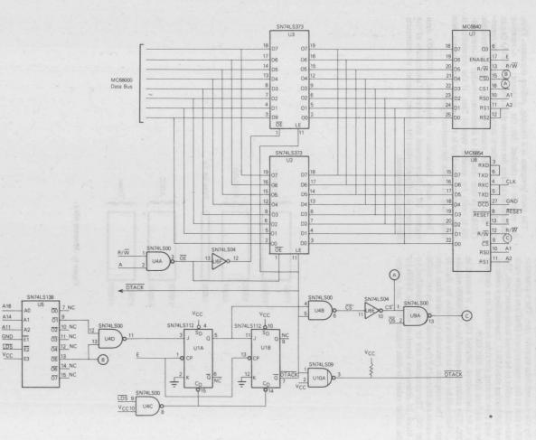
Figure 5. MC68000/MC6840/MC6854 Circuit Example
