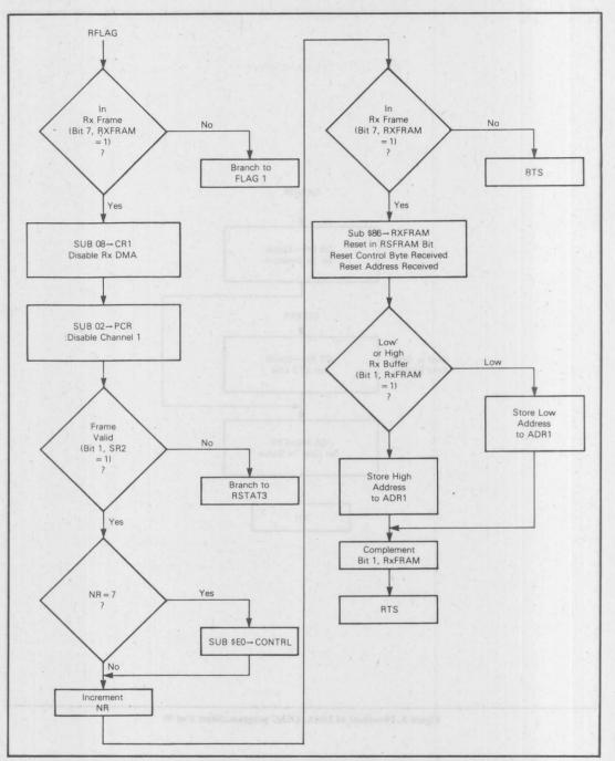
Figure 9. Flowchart of DMA-ADLC Program (Sheet 8 of 9)
