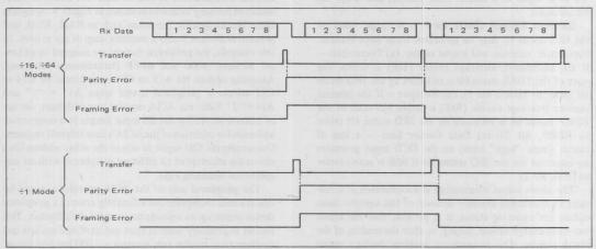
FIGURE 7 – Parity and Framing Errors
