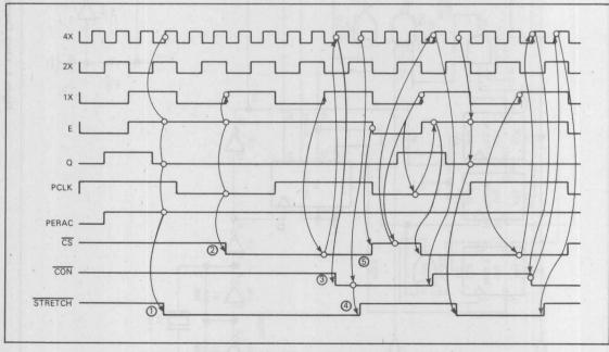
Figure 6. 1 MHz Peripheral Double Byte Access Timing Diagram
