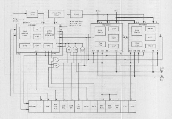
FIGURE 8 - Processor Logic Diagram
