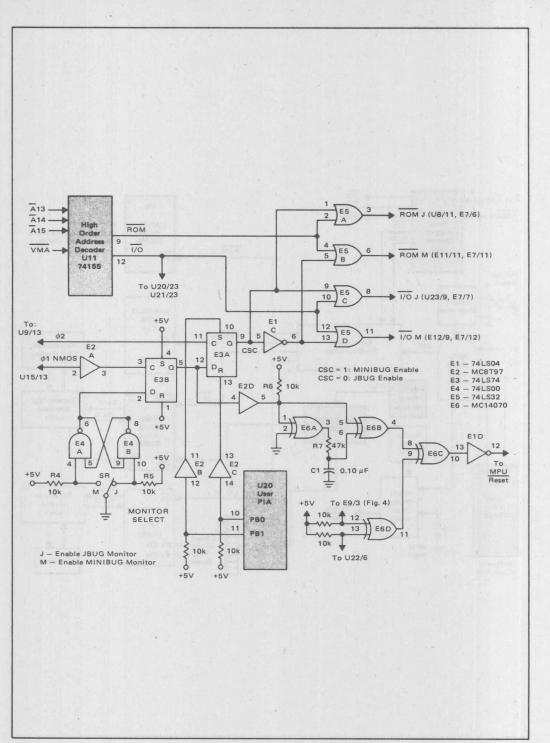
FIGURE 12 - Dual-Monitor Switching Logic
