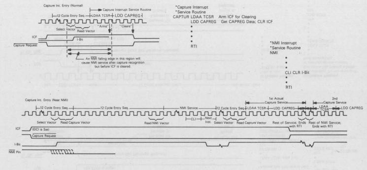
FIGURE 8 Clearing I-bit during <u>NMI</u> service can lead to double service of <u>IRQ1</u> or <u>IRQ2</u> interrupt.
