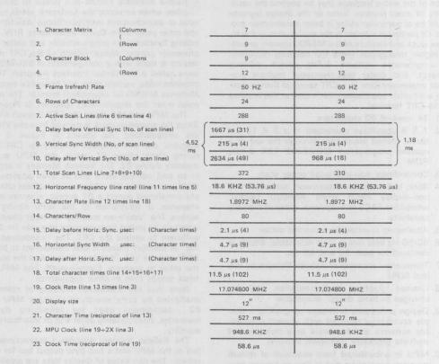
Figure 2 Video Monitor Timing (Motorola Display Products M3000 Monitor meets these requirements)
