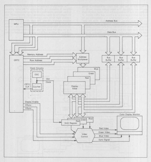
Figure 2. Color Graphics System — Block Diagram
