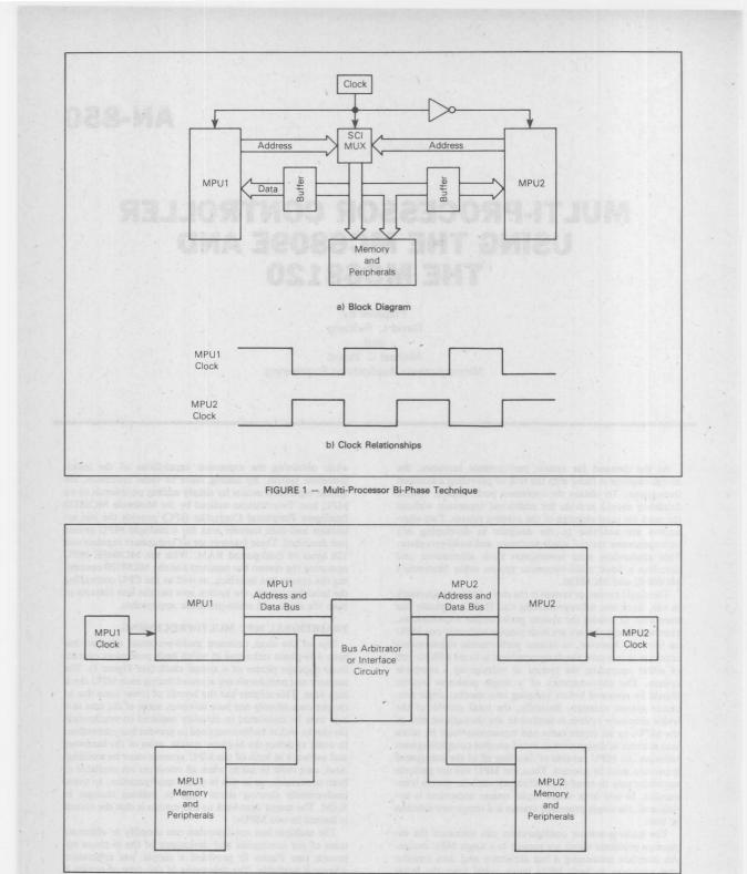
FIGURE 2 - Multi-Processor Multiple Bus Technique (Asynchronous Clocks)
