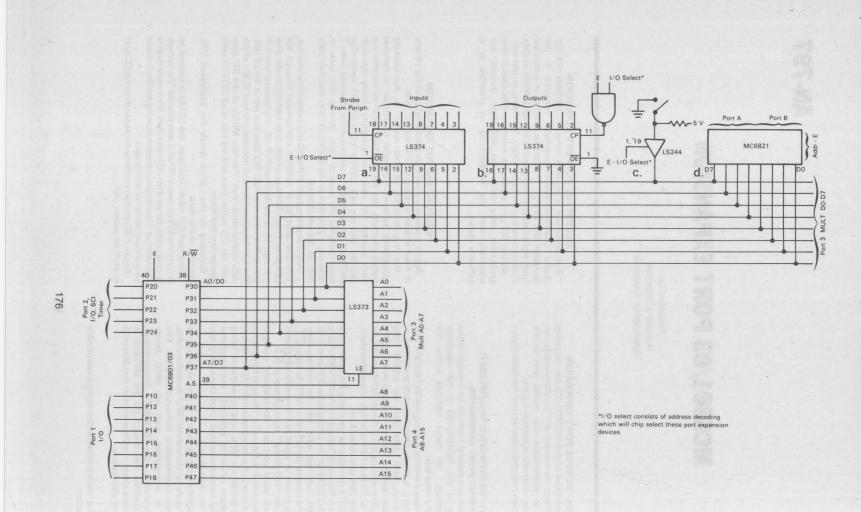
FIGURE 1 — MC6801/MC6803 Expanded Multiplexed Mode Port Expansion
