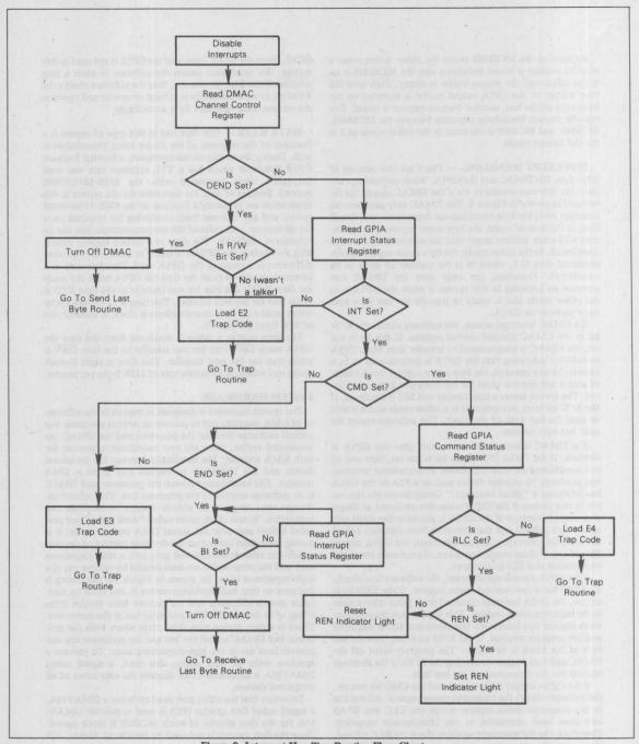
Figure 9. Interrupt Handling Routine Flow Chart
