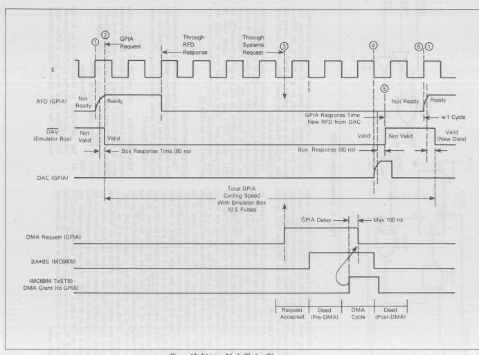
Figure 13. Listener Mode Timing Diagram
