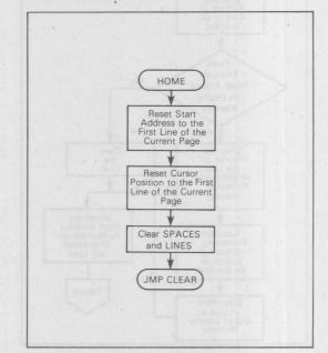
FIGURE 21 — HOME Subroutine Flowchart Reset start address and cursor position to the beginning of the current page, then clear SPACES and jump to CLEAR to put blanks in each display memory element of the current page.
