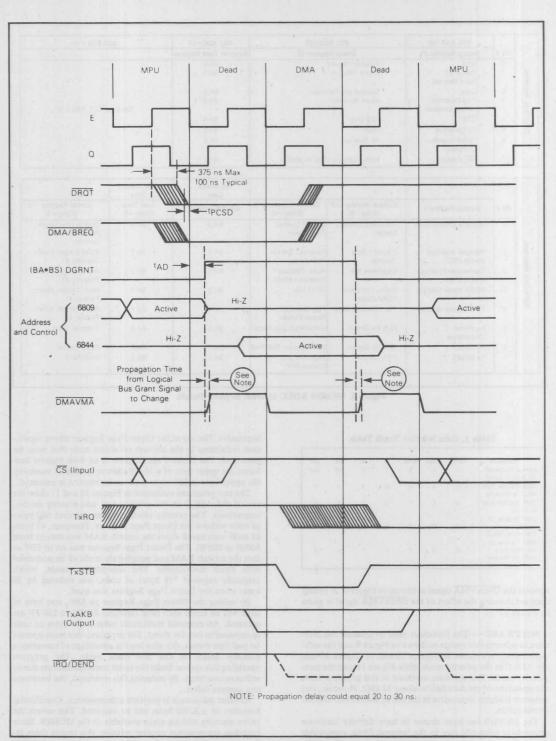
Figure 7. Three-State Steal DMA Timing
