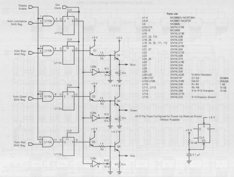
Figure 4. Color Graphics System Schematic (Sheet 3 of 3)
