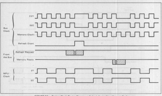
FIGURE 9A - System Clock Timing Diagram - Refresh Cycle, Slow Memory Cycle
