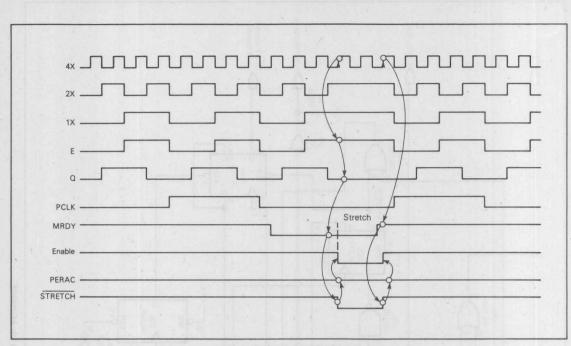
Figure 5. MRDY Timing in MC6809E Clock Generator
