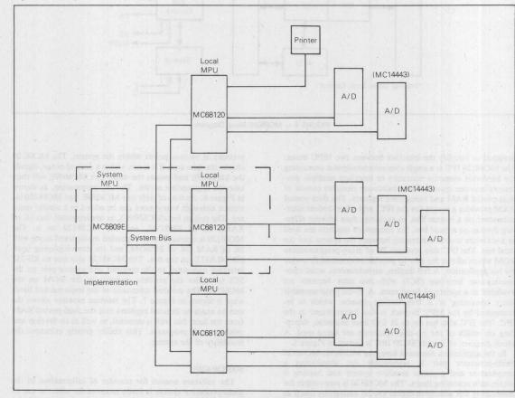
FIGURE 3 — Typical System Configuration
