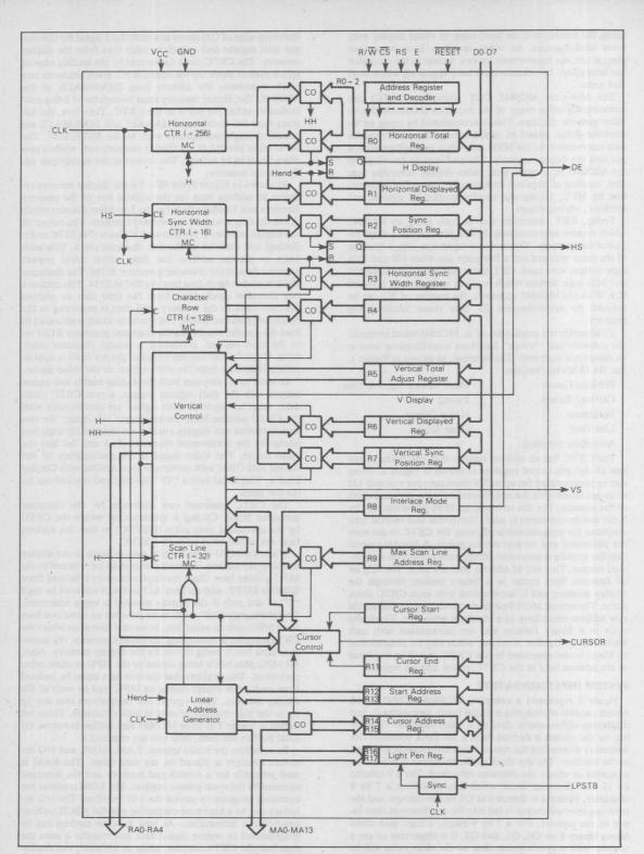
FIGURE 2 – MC6845 CRT Controller Block Diagram
