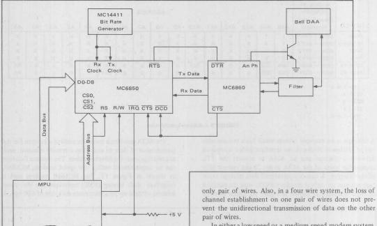
FIGURE 12 - ACIA to Modem Interface
