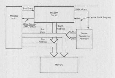
FIGURE 1. Block Diagram Showing DMAC Used in System
