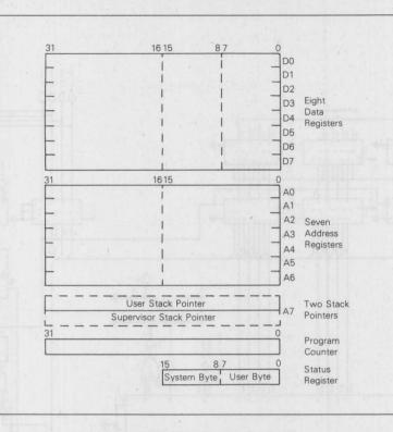
Figure 3. MC68000 Programming Model
