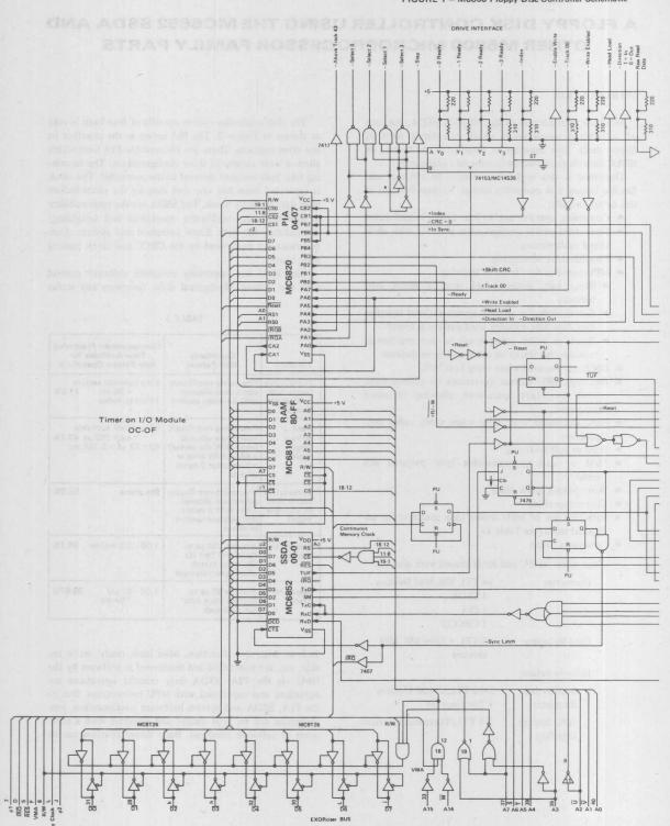
FIGURE 1 - M6800 Floppy Disc Controller Schematic
