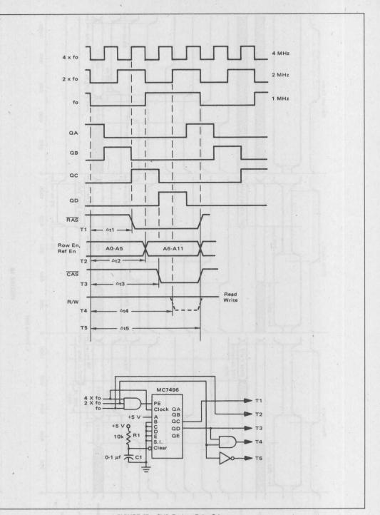
FIGURE 17 - Shift Register Delay Scheme
