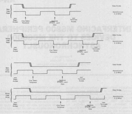
Figure 2. Asynchronous Interface Access Timing Diagrams
