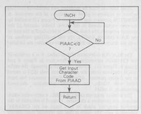
FIGURE 14 — INCH Subroutine Flowchart Polls PIA A Control Register until IRQA1 is set, then the data is retrieved from the PIA A Data Register.
