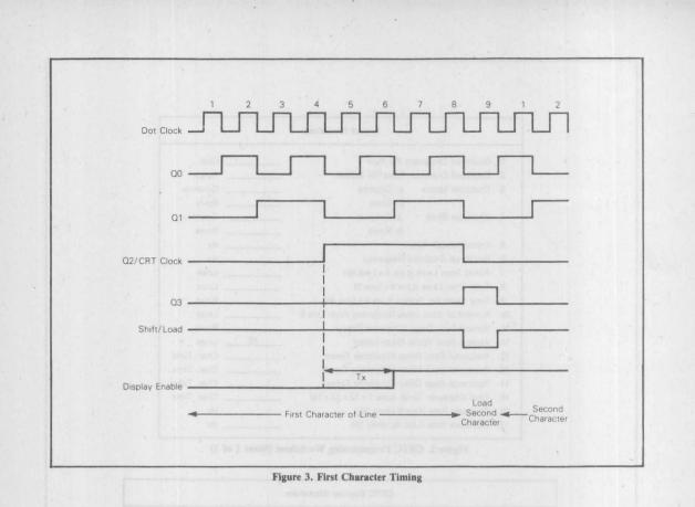
the first character row, increments the row address by one, and then steps through the same addresses again. This procedure is repeated until the row address is equal to the address contained in the maximum scan line address register. The row address is reset to zero and the second character row is displayed.
