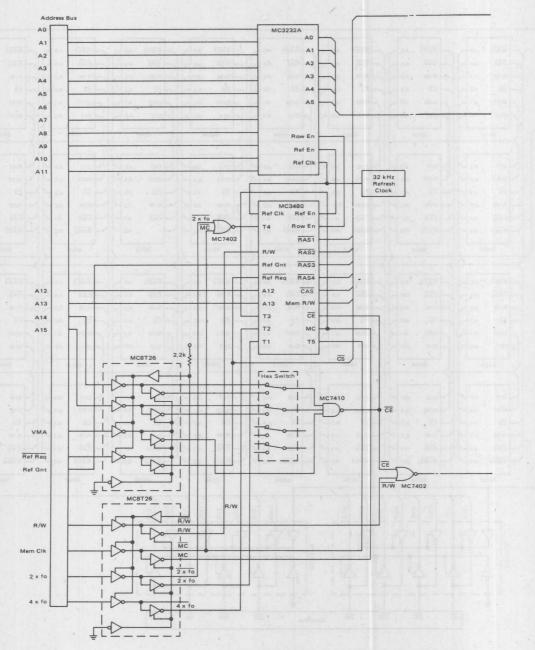
FIGURE 18 - 16K Dynamic RAM Using 4 fo and 2 fo Timing
