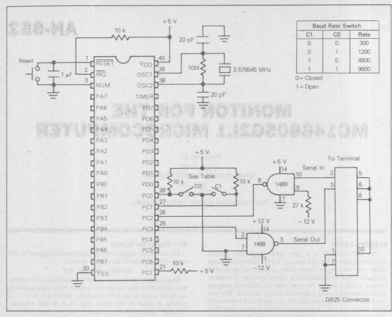
FIGURE 1. Monitor Mode Schematic Diagram
