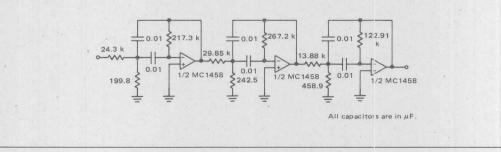
FIGURE 14a - Originate Filter Component Values
