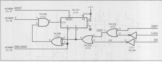
**Figure 12. Synchronization Circuitry**
