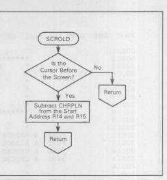
FIGURE 22 — CLEAR Subroutine Flowchart Stores ASCII blank, code \$20, into all memory locations on the current page starting at the cursor. FIGURE 23 - SCROLD Subroutine Flowchart
