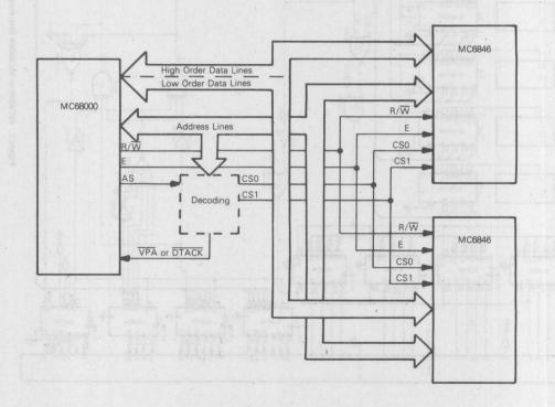
Figure 1. MC6846 to MC68000 Interface - Block Diagram
