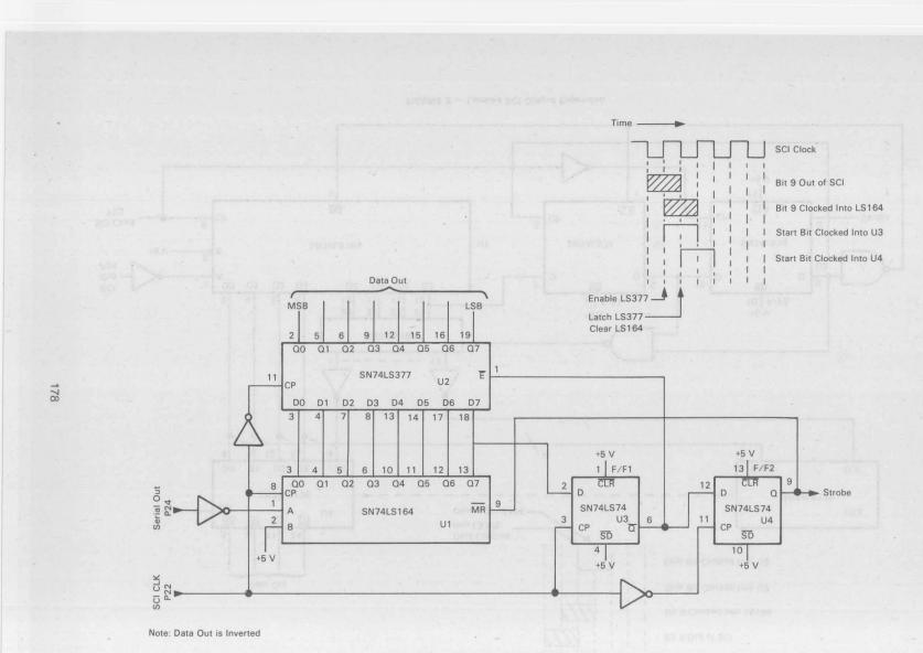
FIGURE 3 — SCI Latched Port Expansion
