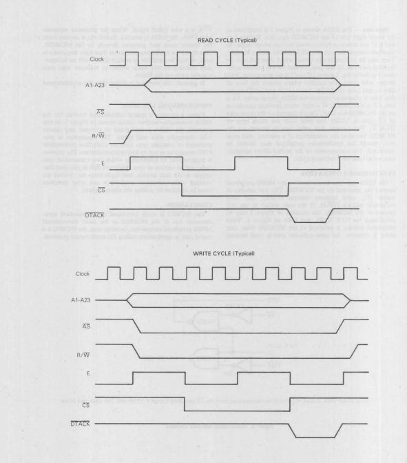
Figure 2. MC68000/MC68B52 Interface — Timing Diagrams
