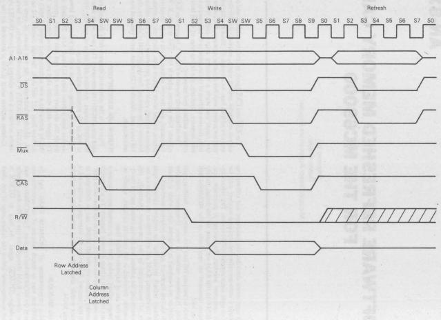
Figure 1. Read, Write, and Refresh Timing Diagrams
