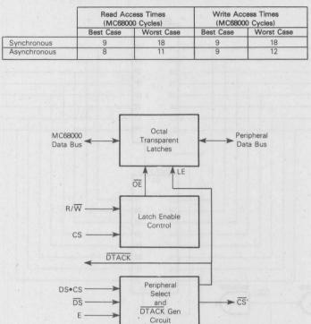
Table 1. Synchronous and Asynchronous Interface Access Time
