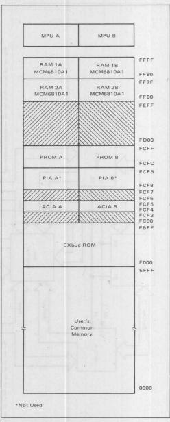
FIGURE 4 - Dual Processor System Memory Map
