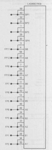
Figure 4. Liquid Crystal Display (LCD) Connections
