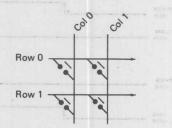
A non-encoded keyboard is a set of switches wired in a column/row matrix.
