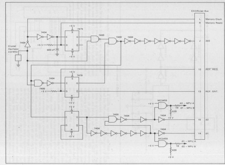
FIGURE 8 - System Clock Schematic
