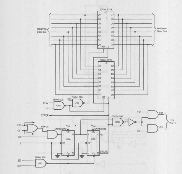
Figure 5. Asynchronous Interface Circuitry
