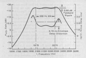
FIGURE 14b - Originate Filter Gain and Group Delay
