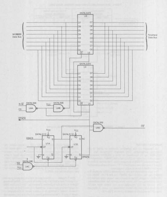
Figure 4. M6800 Peripheral to MC68000 Interface - Schematic Diagram
