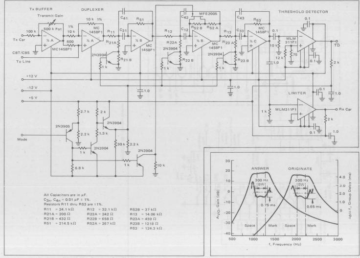
FIGURE 17a - Switchable Filter/Duplexer
