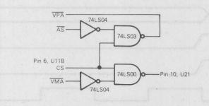
Note: When VMA is used, AS should be disconnected from the CS decoding (Figure 1, U11B) and that input tied active.
