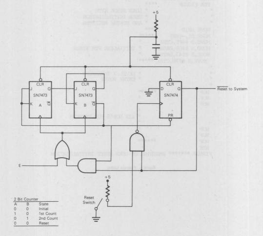
Figure 4. Vectored Interrupt Circuit - Schematic Diagram
