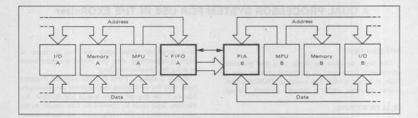
FIGURE 2 - Dual Processor System Using a FIFO
