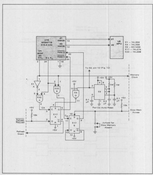
FIGURE 4 - Memory Control Handshake Logic
