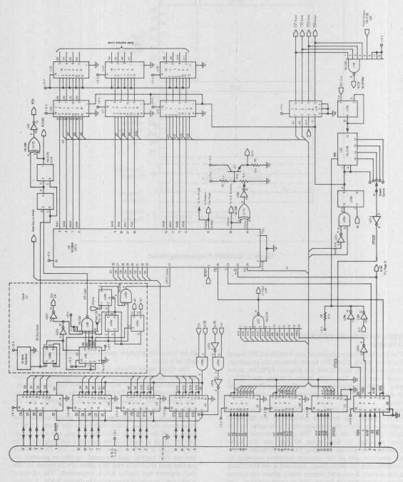
Figure 4. Color Graphics System Schematic (Sheet 1 of 3)
