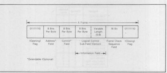
Figure 5. Data Format of a Message Frame
