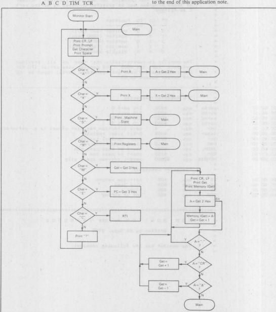
FIGURE 2. Monitor Mode Operating Flowchart
