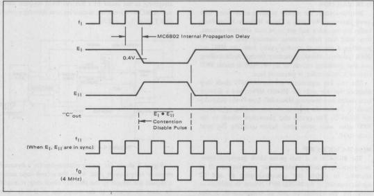
FIGURE II - Dual MC6802 Synchronizer Timing
