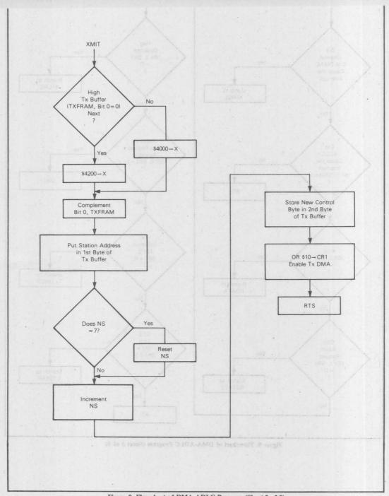
Figure 9. Flowchart of DMA-ADLC Program (Sheet 2 of 9)
