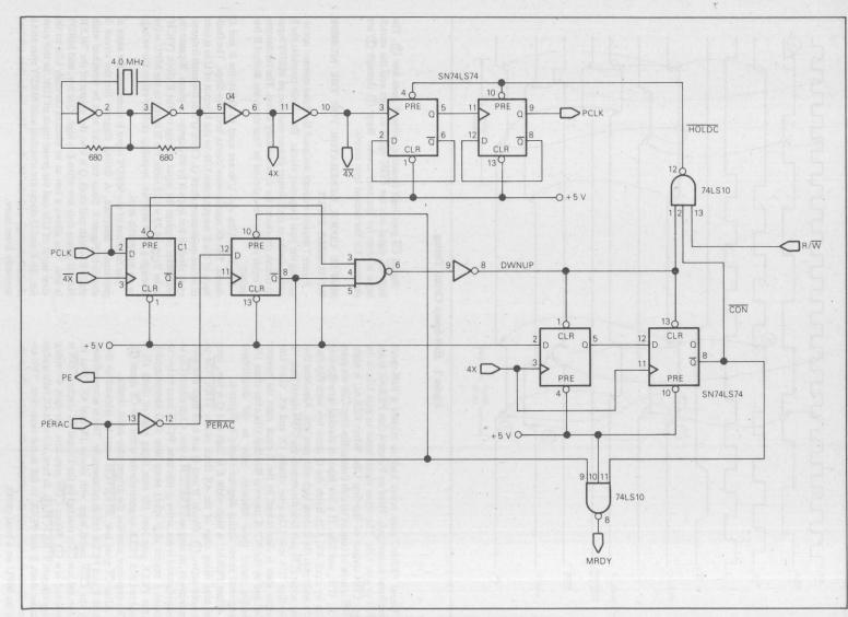
Figure 2. MC6809 Half-Speed Peripheral Clock Circuit
