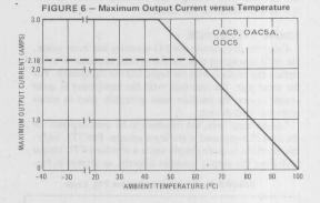
Since the input modules are not power-handling devices, they do not have a derating factor and may be used over the specified temperature range without derating.
