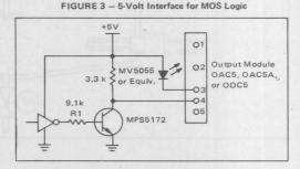
of an NPN transistor, which, in turn, drives the output module. By changing the value of R1 to  $39 \text{ k}\Omega$ , this configuration may be used to interface CMOS operating at 15 volts with 15-volt logic modules OAC15, QAC15A, and ODC15.
