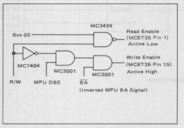
FIGURE 12 - Bus Control Logic
