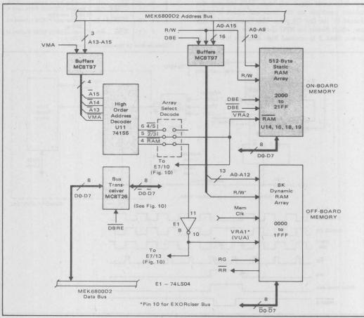
FIGURE 8 – Addressing for 8.5K Memory Configuration
