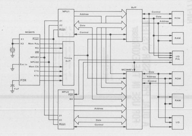
FIGURE 22 - Dual Processor (DMA) Using Halt
