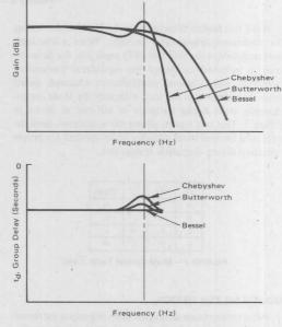
FIGURE 10 - Filter Approximation Characteristics
