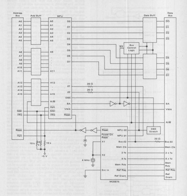
FIGURE 10 - Block Diagram
