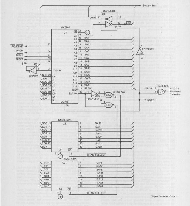
Figure 4. MC68000 Sequential Memory Byte Transfer Interface System
