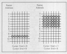
FIGURE 8 - Cursor Start and End Register
