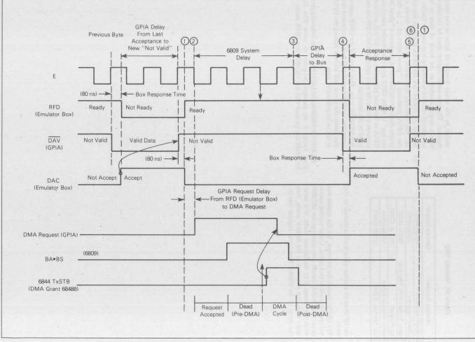
Figure 14. Talker Mode Timing Diagram
