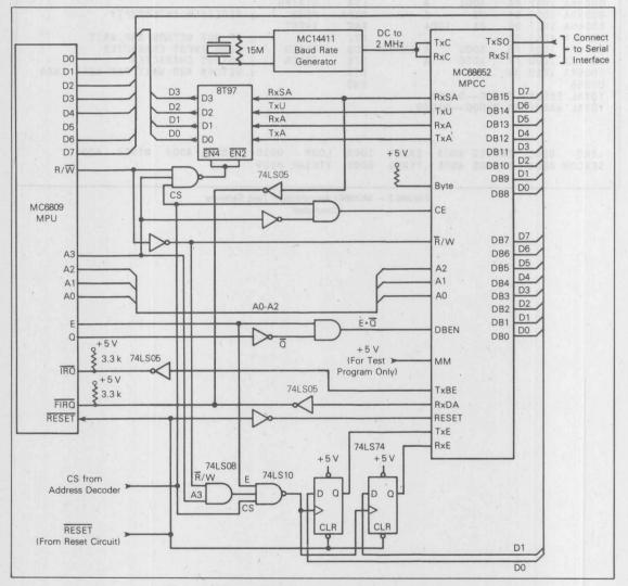
FIGURE 3 - MC6809 to MC68652 Interface Connection, Schematic Diagram
