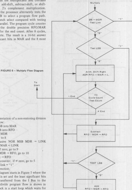
Divide is an implementation of a non-restoring division algorithm as shown below:
