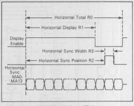
FIGURE 5 - Horizontal Timing
