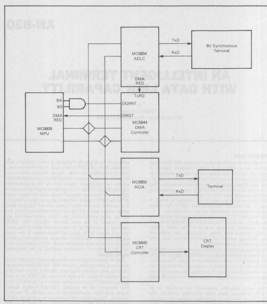
Figure 1. Intelligent Terminal - Block Diagram
