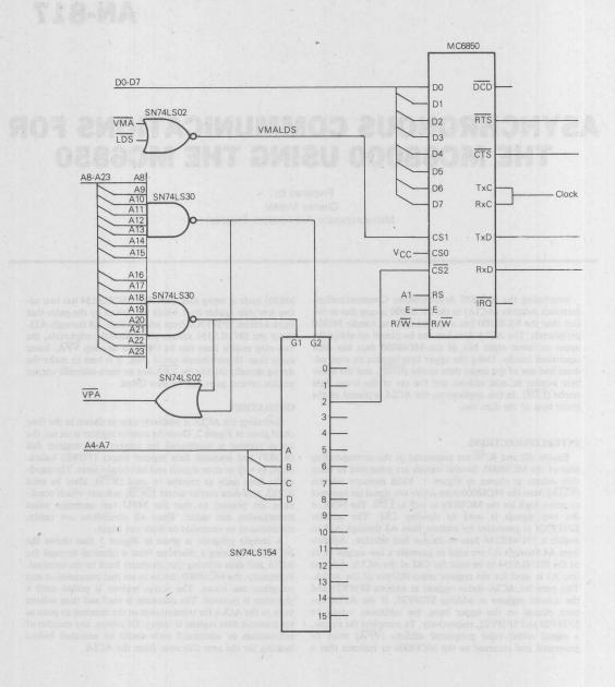
Figure 1. MC6800 to MC6850 Interconnections
