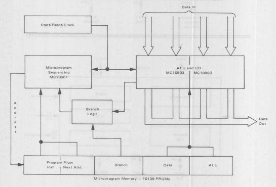
FIGURE 2 - Processor Block Diagram
