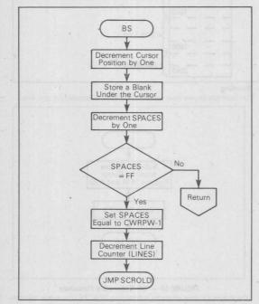
FIGURE 18 – BS Subroutine Flowchart Backspaces and blanks under cursor. Jumps to SCROLD and checks
