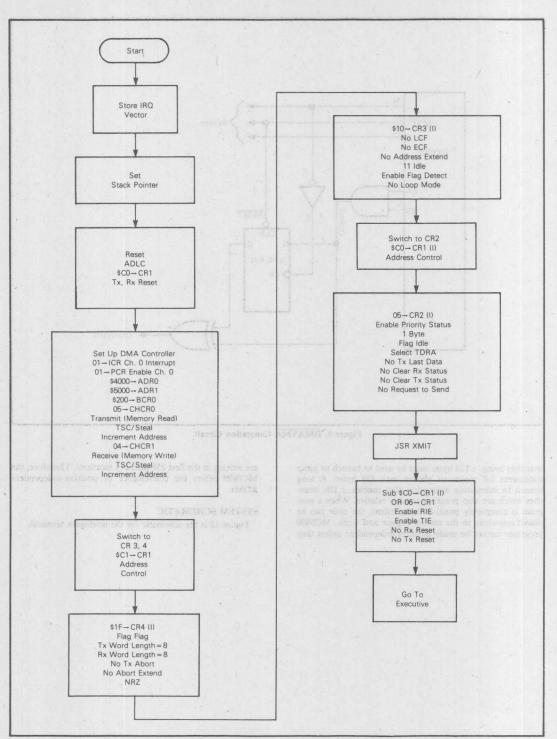
Figure 9. Flowchart of DMA-ADLC Program (Sheet 1 of 9)
