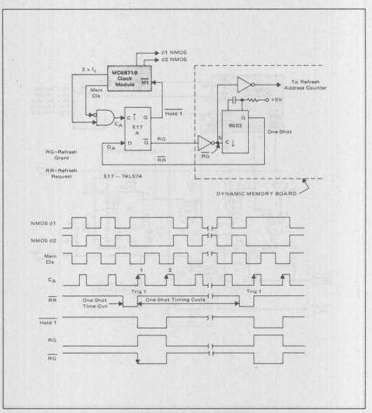
FIGURE 5 - Memory Refresh Handshake Logic and Waveforms
