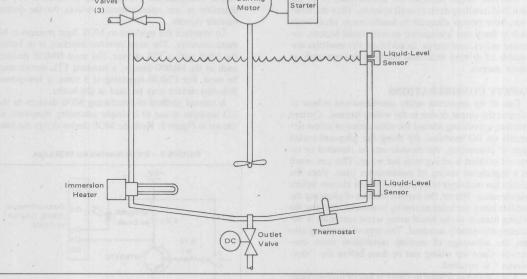
in a plant that batch-processes liquids through a number of mixing, stirring, and heating cycles. The original plant was controlled by relay logic and had high operating cost due to direct operating labor and maintenance expense. The goal of the conversion of the plant to a distributed processor-based control system was to increase flexibility while increasing reliability and reducing labor.
