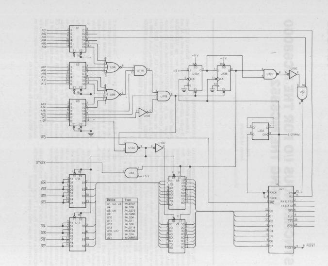
Figure 1. MC68000/MC68B52 Interface - Schematic Diagram
