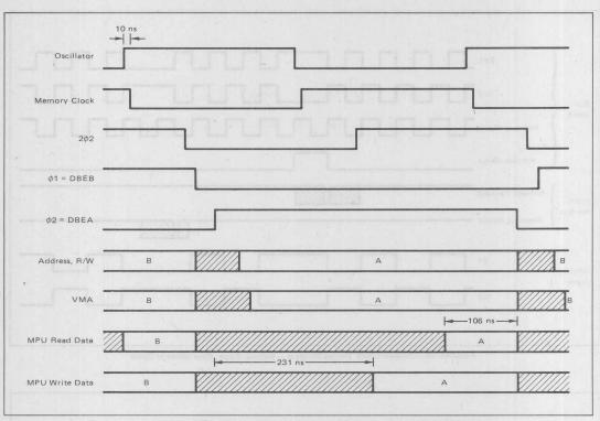
FIGURE 9C - System Clock Timing Diagram - Data Transfer To and From MPU
