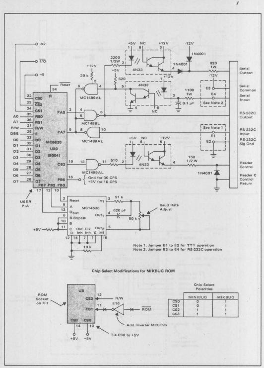
FIGURE 18 - Terminal Interface Logic for MIKBUG
